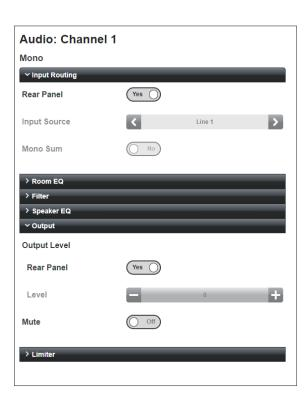
The EQ sections have "basic" (2-band) and "advanced" (7-band fully parametric) modes.
