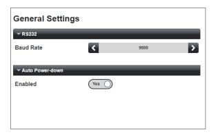
Selectable baud rate option: 4800, 19200, 38400, 57600 and 115200 (default 9600) and Auto power-down can be disabled, for example, in paging- or announcement-only applications, where an immediate response to an input signal is required. With Auto power-down disabled, the CVA amplifier will nolonger go into standby mode due to lack of input signal activity
