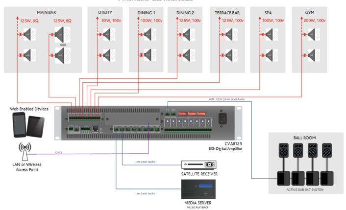
The example above shows an how the eight channels of a CVA8125 amplifier may be used to provide audio to different areas of a hotel with a Club facility.
