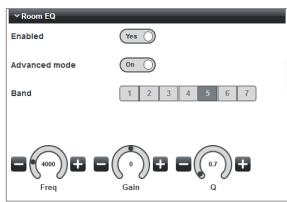
Audio channel configuration allows expanded input routing options, stereo-to-mono summing, room and loudspeaker EQ adjustment, limiting and output level control. This page also allows the configuration of the output mode of the amplifier channels.
